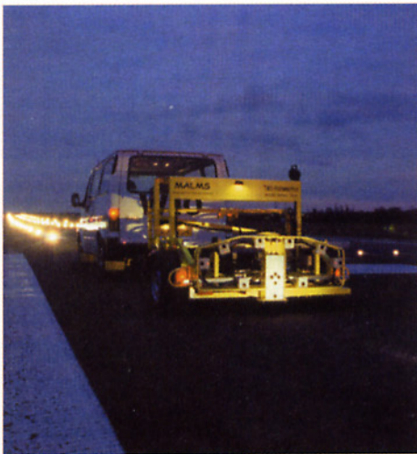
THE TRAILER-MOUNTED MALMS SYSTEM CAN TEST LIGHT OUTPUT AT 50 MPH.
